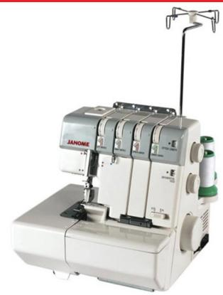
The Pro 4 DX makes serger sewing easy! Incorporating the differential feed system of two feed dogs, puckered edges on woven fabrics and stretched edges on knits are virtually eliminated. The rolled hem conversion feature eliminates the need to change the needle plate, foot, or tension setting for rolled hemming. Restructured lower looper guides allow easy access. The included threading card and color-coded guides are easy to follow for 2, 3, or 4 thread serging.
